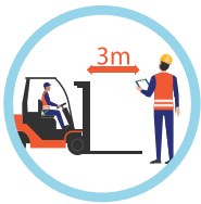
Separate People and Mobile Plant
